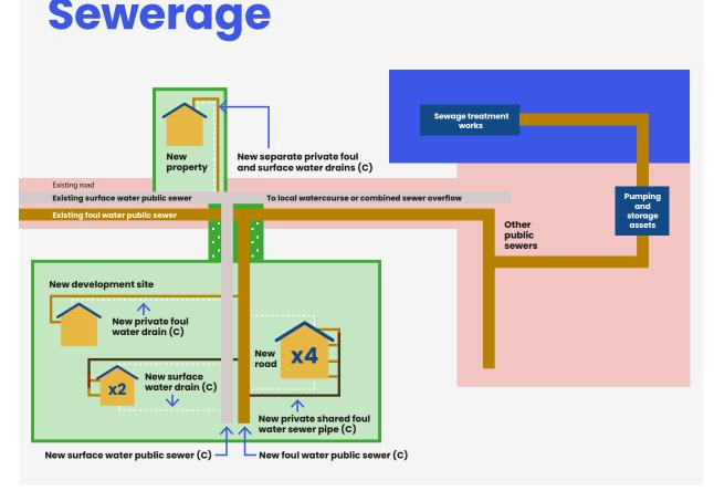
We've left surface water sewerage out of this diagram to make it easier to read, but you can still request this infrastructure, and discharge would be made to a suitable outfall.
