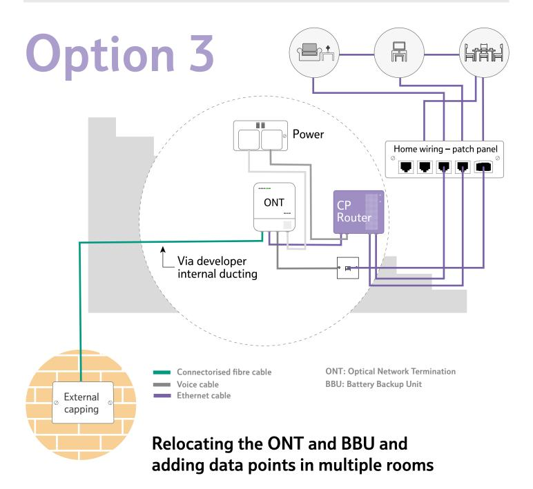
As per option 2 this extends the number of fixed sockets so that the home owner doesn't need to rely on wireless connections in the majority of the house. This would enable the down-streaming of 4K television in those areas where the customer is most likely to use high bandwidth applications like streaming TV, gaming consoles or video conferencing.
