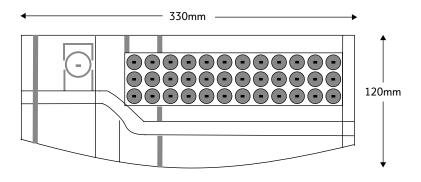
Array of ports for internal fibre cable located at bottom of fibre DP/splitter
