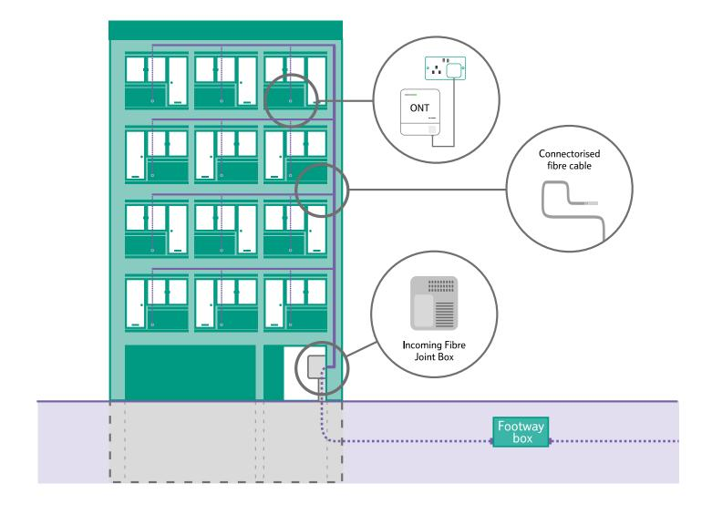
Openreach will create a fibre layout based on your Mechanical & Electrical (M&E) drawings (on larger MDUs) of the MDU. The design will calculate the stores required to build the network.
