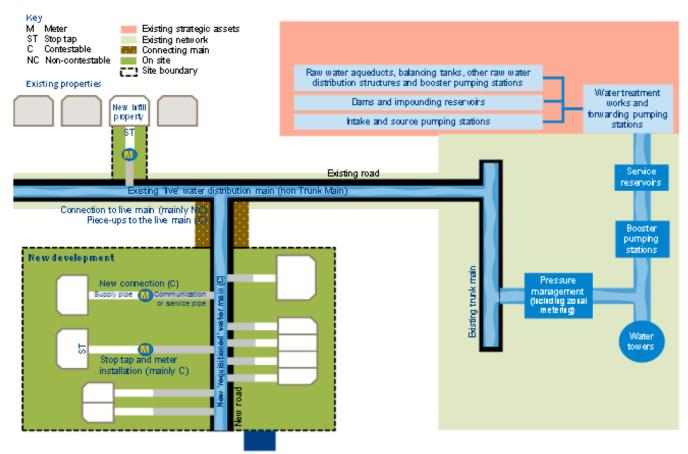
C – Contestable Works which are able to be undertaken by others NC – Non Contestable Works which are to be undertaken by Water Company only
